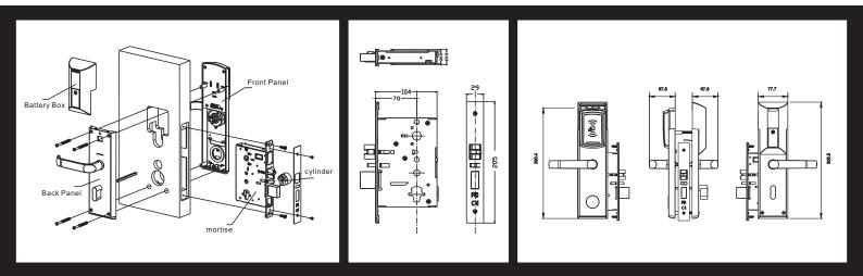
Features:Bright,Magnificent,Durable,Reliable Material:Zinc Alloy+Stainless Steel Finish option:CCR,PVD Mortise option:M1,suitable for ≥38mm thickness doors M3,suitable for ≥28mm thickness doors
